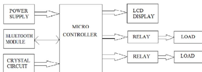
Figure .1Process of Bluetooth home automation device
