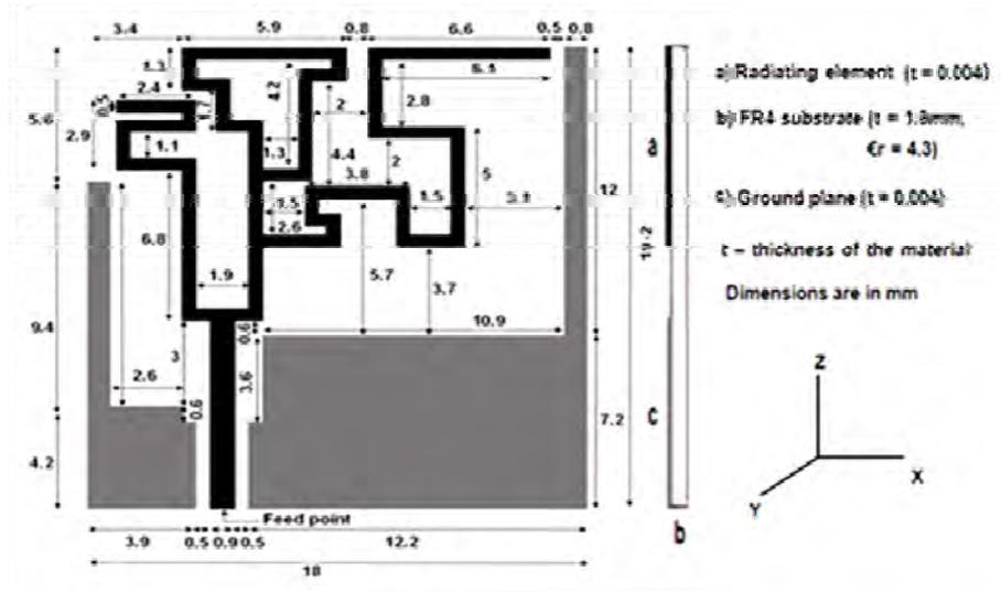
Figure 1. Geometry of the Z-U-T-S shaped antenna front and side view
