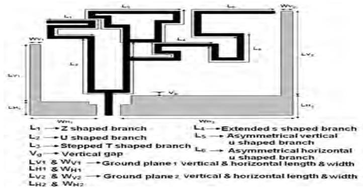
Figure 3. Parameters of Z-U-T-S shaped antenna
