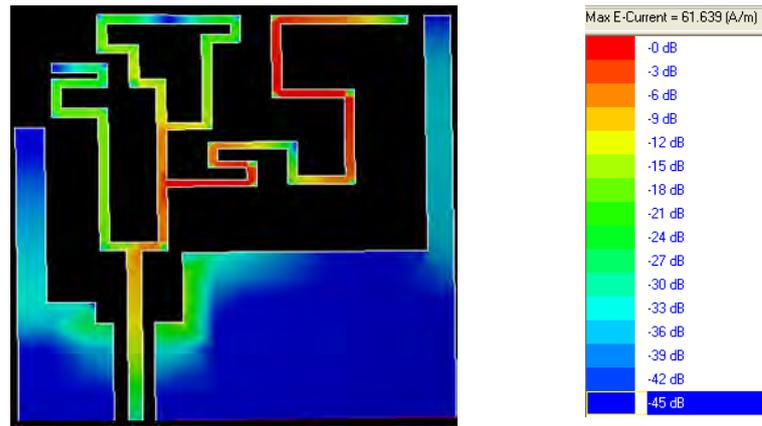
Figure 6 (b) Surface Current Distributions at 6.3GHz
