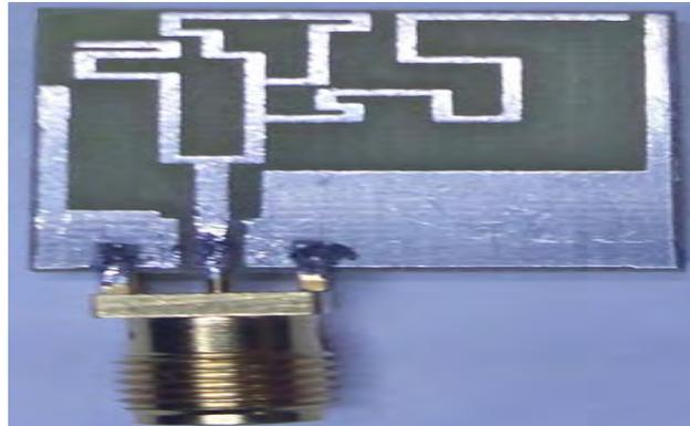
Figure 2. Fabricated Z-U-T-S shaped antenna
