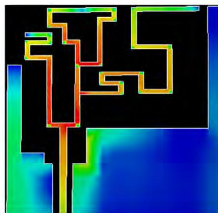
Figure 6 (a).Surface Current Distributions at 4.6GHz
