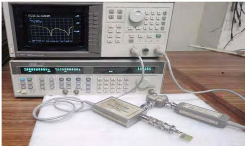
Figure 5. Return loss measurement using HP 8757D Scalar Network Analyzer for a Z-U-T-S shaped antenna.
