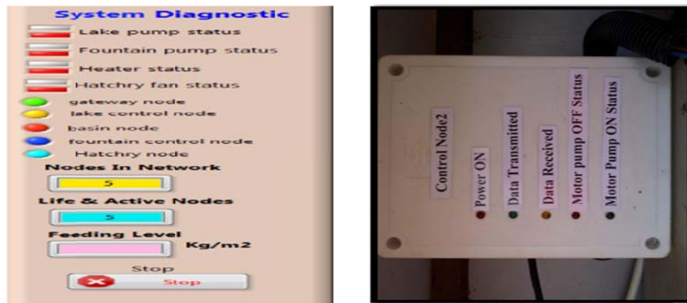
Figure 11 Diagnostic subsystems and control Node2 diagnostic LED
