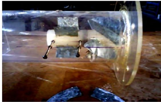
Fig.1 Eight Rotating vane swirler with guide vane at  $0^\circ$  inlet and  $0^\circ$  outlet angle
