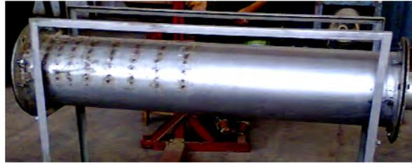
Fig. 3 Expansion chamber
