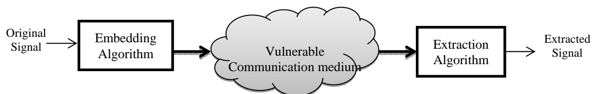
Figure 1. General Framework of Watermarking System
