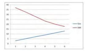
As we can see graphs show, there is inclide curve of MSE with increase of size of window and decline curve has been observed in case of PSNR. Similar observation has be noticed in case of SNR courves with window size.
