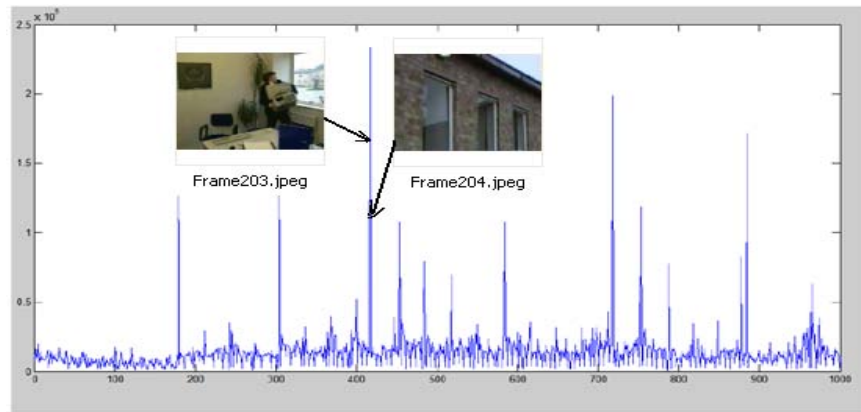
Figure 2 Hue-Histogram Difference graph for key frame detection with two different consecutive frames having maximum difference.
