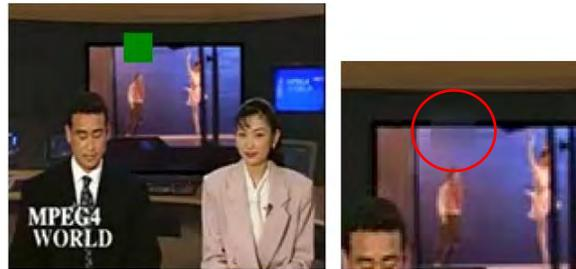
Figure 7. Blocking artifacts due to bilinear interpolation
