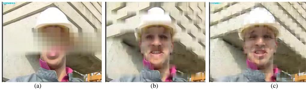
Figure 4. FMO performance on *Foreman* frame 10. (a) Raster scan (no FMO). (b) Interleaved FMO. (c) Dispersed FMO.
