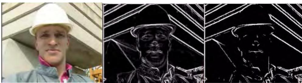
Figure 8. Applying Sobel operator to (left) *Foreman* frame, (middle) all detected edges, (right) prominent edges with threshold of 100
