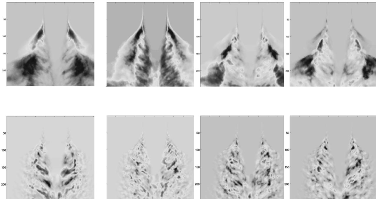
Figure 2: Comparison of first 4 POD modes (top) and DMD modes (bottom) for medium pressure LES gas jet concentration field.
