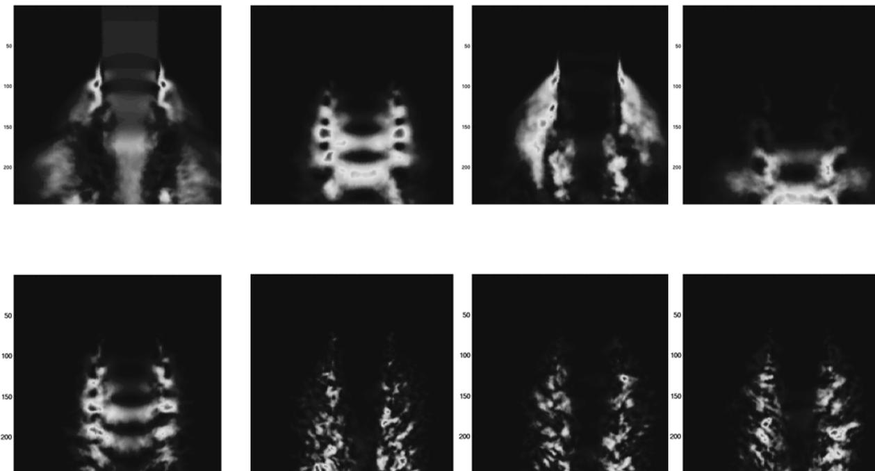
Figure 4: Comparison of first 4 POD modes (top) and DMD modes (bottom) for medium pressure LES gas jet velocity field.
