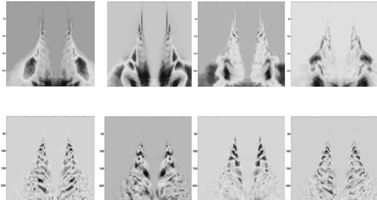
Figure 1: Comparison of first 4 POD modes (top) and DMD modes (bottom) for low pressure LES gas jet concentration field
