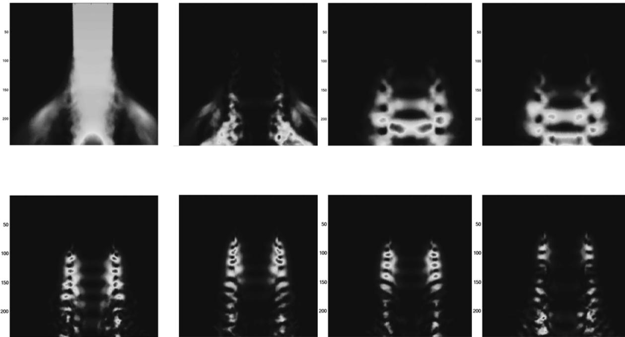
Figure 3: Comparison of first 4 POD modes (top) and DMD modes (bottom) for low pressure LES gas jet velocity field.
