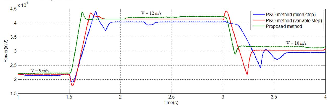
Figure 9. Simulated dynamic response of WECS output power due wind speed step change.
