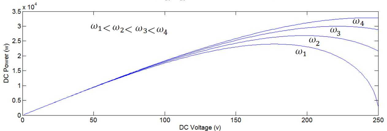
Figure 4. Typical rectified power versus rectified voltage.
