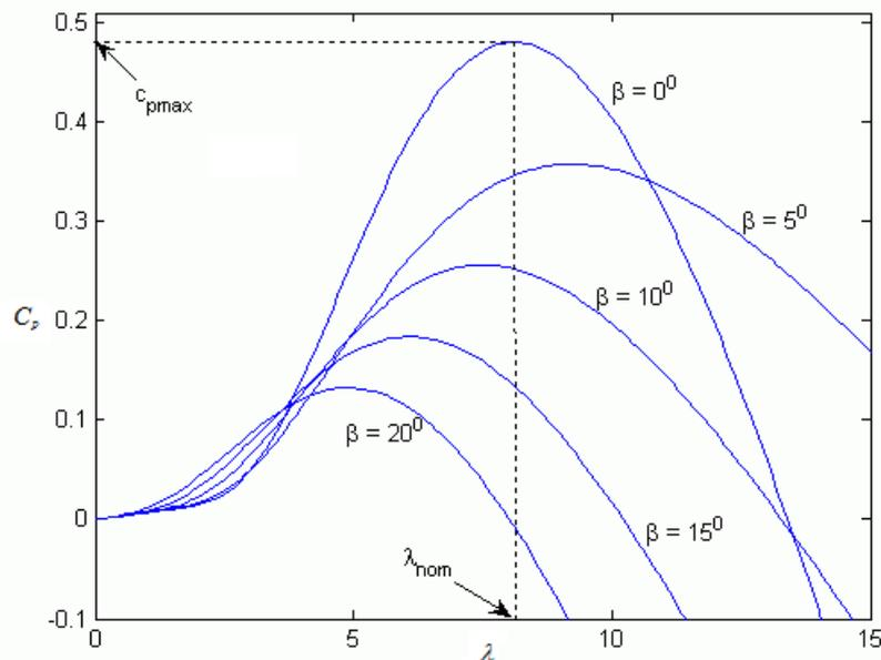
Figure 2. Typical  $C_p$  versus  $\lambda$  curve.
