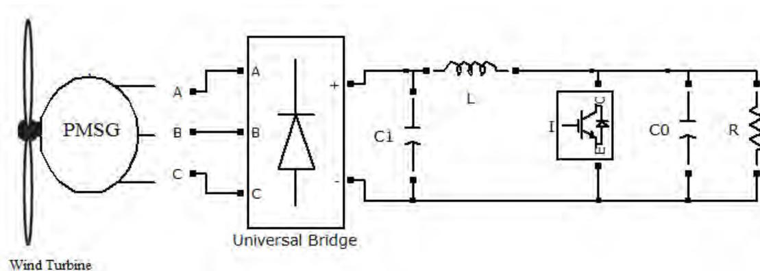
Figure 1. Wind generator system.
