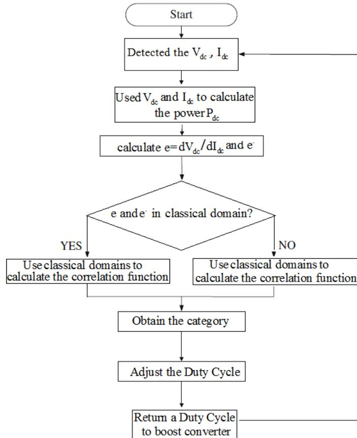
Figure 7. The Flowchart of the Extension MPPT Algorithm.
