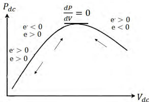
Figure 6. The P-V Curve Slope of Error and Change of Error.
