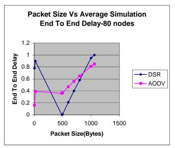
This graph shows that average simulation end to end delay of DSR goes on increasing as the packet size increases.
