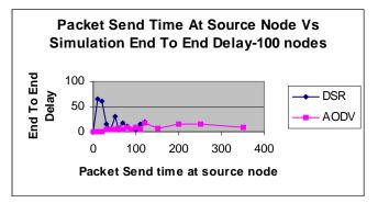
Here we observe that the end to end delay of DSR is greater than AODV. 3-Packet Size Vs Average Simulation End to End Delay
