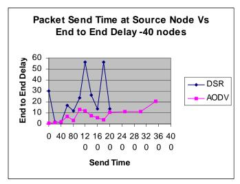
2-Packet send time at Source node Vs. Simulation End To End Delay
