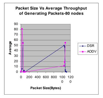
One can clearly notice that the average throughput of generating packets for AODV increases as the packet size keeps increasing.
