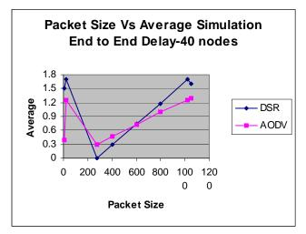
From this we observe that the average simulation end to end delay of DSR is increasing as the packet size is increasing.
