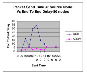
Here we observe that the end to end delay of DSR is much greater than AODV.
