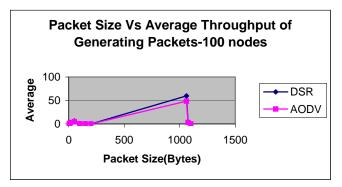
From this graph we observe that as the packet size is increasing the average throughput of generating packets for DSR is slightly greater than AODV.
