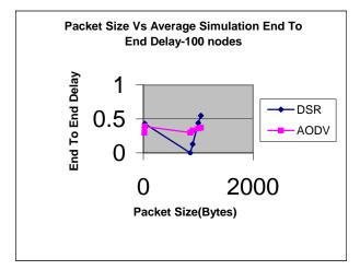
This graph shows that as the packet size is increasing the average simulation end to end delay of DSR increases and is greater than AODV.
